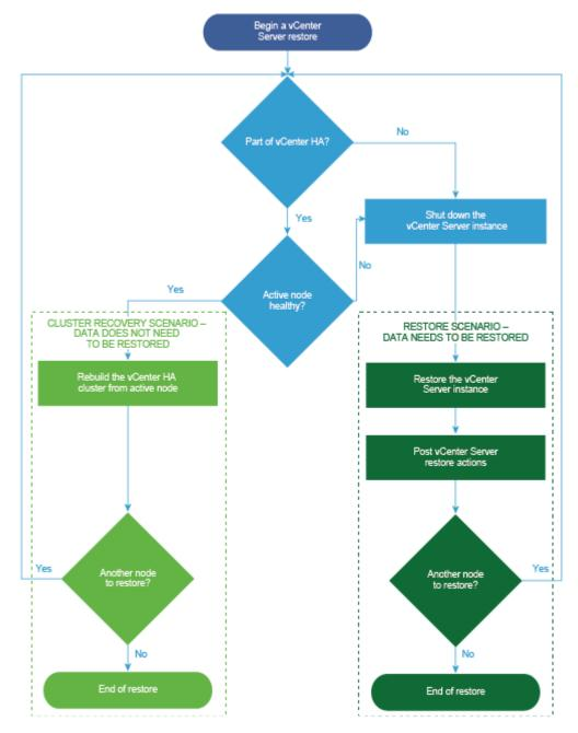
Figure 8. vCenter server restore workflow
